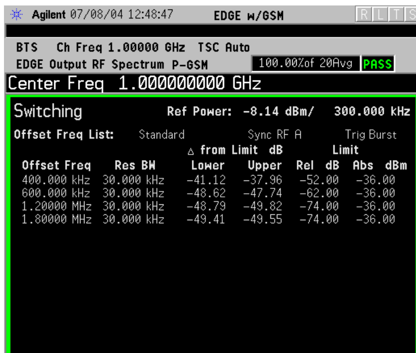
Figure 2-14 EDGE ORFS Result - Switching Margin & Limits View
